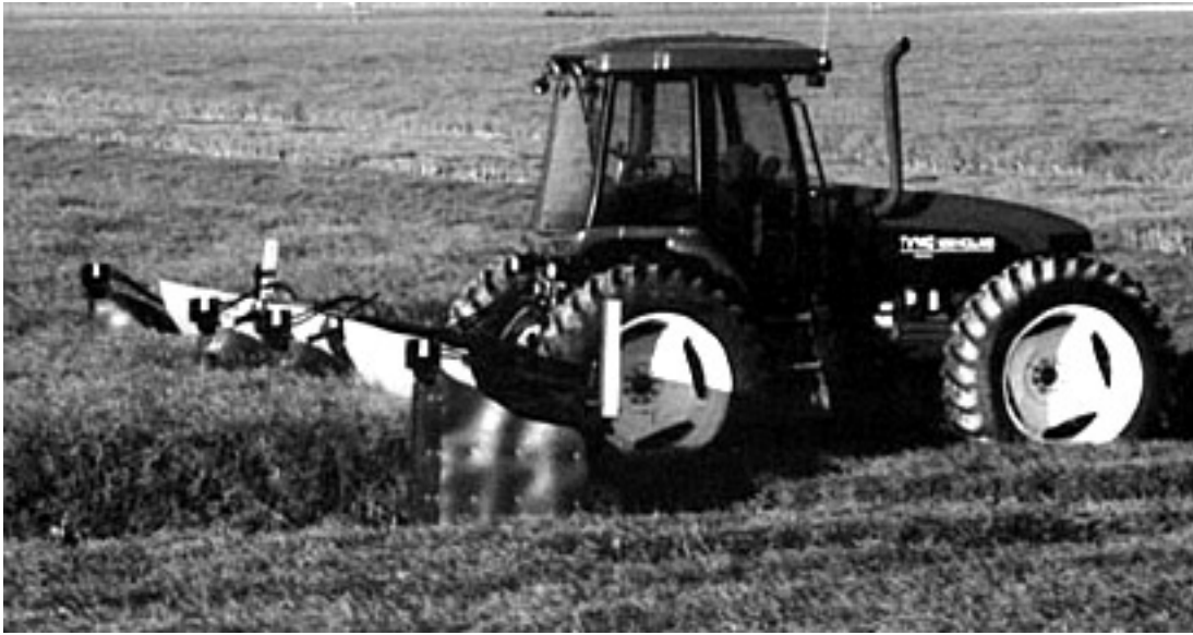
Figure 1. The Yield Shield from AgShield of Canada is used to bend canola stalks while green, which the company claims encourages a more uniform ripening of seed without cutting the plant. Note: The steering mechanism on the tractor swivels, so it is actually driving backwards!
