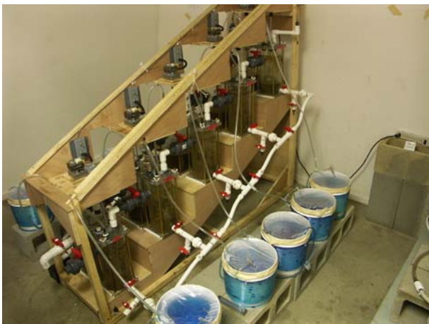
5 in a series anaerobic digester reactor
